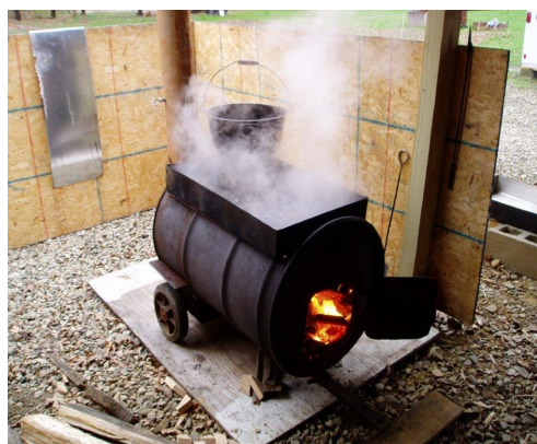
Figure 15. Boiling sap on a barrel stove with a preheating pan.
